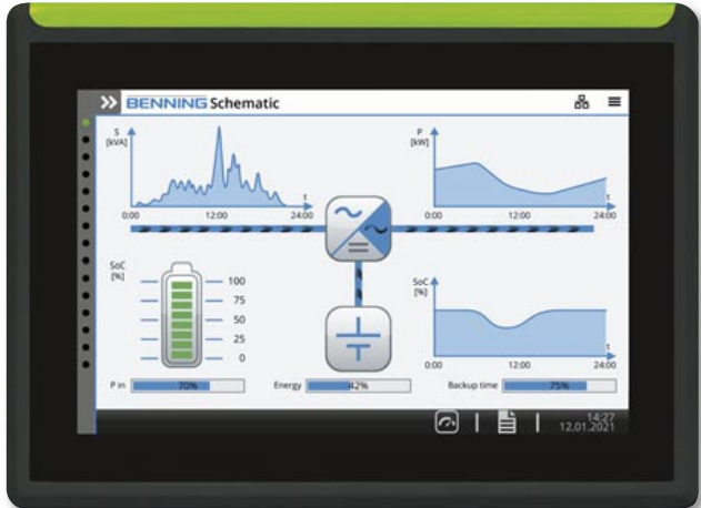
Figure 8: The Monitoring and Control Unit (MCU) supports a range of protocols and interfaces for connecting the system EMS from the widest range of software manufacturers. The MCU 3000 system controller, which is installed in the cabinet door of the power supply system, has a 10.4" touchscreen.
